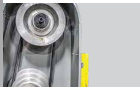
4 SPEED STEP PULLEY BLADE DRIVE
