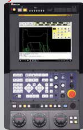
◀ CAM ON BOARD The on board CAM and interactive software support various grinding processes. The 15" touch panel is positioned at the same height as the main motor allowing a smooth working environment.
