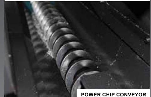
POWER CHIP CONVEYOR
