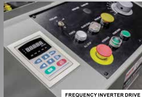
FREQUENCY INVERTER DRIVE
