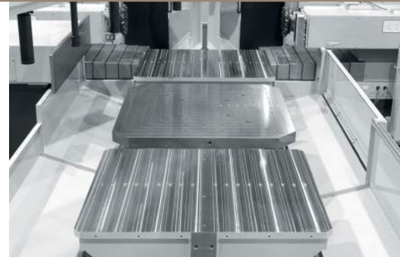
Material Support with Patent-Registered Indexing Unit
