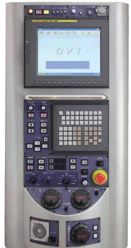
12-inch Color LCD Touch Panel (top) USB Port (above) Operation Panel (right)
