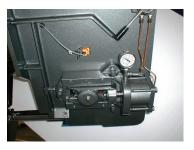
**Blade Tension** is hydraulic and is calibrated to provide accurate cutting and optimum blade life.
