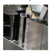
**Split Front Vise Jaws** hold the work securely on both sides of the blade minimizing vibration and burs, while also helping to reduce the remnant length to as little as 3". The full stroke hydraulic vises provide ease of operation and simplify set up.
