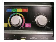
**The Operator Control Panel** is conveniently located at the front of the machine providing the operator with a clear view of the cutting area.
