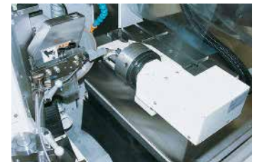
Tool Grinding Combining NC Swiveling Axis
