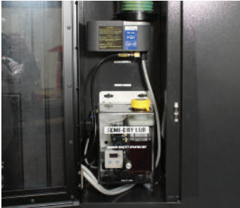
Semi-Dry Lubrication System for Milling
