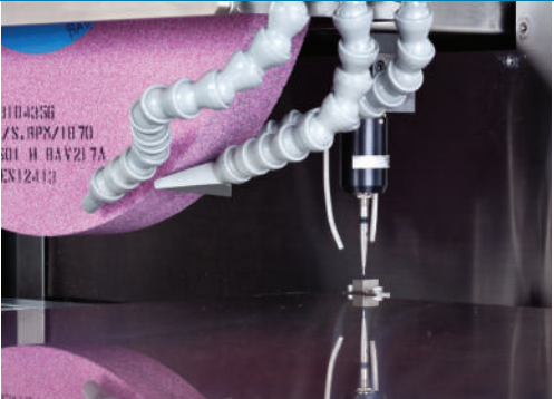
On-Board Measuring Touch Probe
