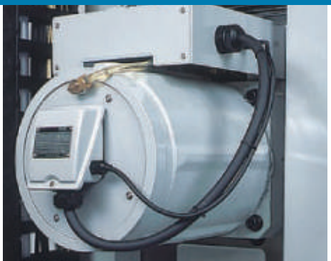
Ultra-Low Vibration Spindle Motor
